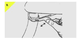
Push the lever 5-10 times to make sure the cable housing is fully seated and to check for play in the cable. Note: If the lever isn't returning, check cable routing to ensure proper installation of the cable. If there is play in the lever/cable, loosen barrel nut with 2mm and 3mm allen wrenches and pull cable tight a second time. For micro adjustment, use the rotary ferrule on the cable housing.
