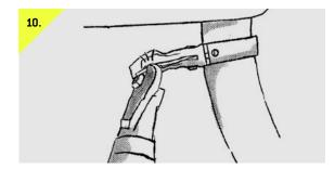
Slide cable into the guide under the lever. Trim excess cable with cable cutters with enough room to place cable end, approximately 10mm. It is important to use proper cable cutters to prevent the cable from fraying.
