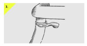
Position lever on bar and clamp in place with a 2.5mm allen wrench to a maximum of 2nm.
