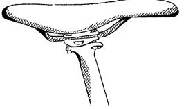
PLACE SADDLE RAILS INTO CLAMP, ADJUST ANGLE AND FORE/AFT POSITION PER BIKE FIT, TIGHTEN BOLTS WITH 5MM ALLEN WRENCH TO 8-10NM.
