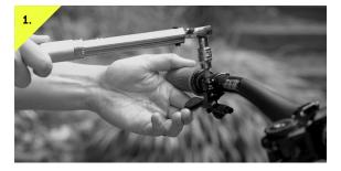
Position hinged clamp on bar and attach lever to clamp using one of the threaded hole options on lever body to achieve your desired position. Tighten with 4mm allen wrench to maximum 4nm. Note: this position can be changed after install to fine tune fit. If using with a sram mmx adapter, install lever to adapter using T25 torx wrench
