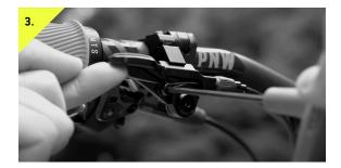
Pull cable tight and torque cable fixing bolt to 2.5 Nm with a 3mm allen wrench. Note: make sure cable is seated underneath the washer to ensure proper cable retention with the washer.
