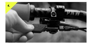
Push the lever 5-10 times to make sure the cable housing is fully seated and to check for play in the cable. Note: if there is play in the lever/cable, loosen cable fixing bolt with 3mm allen wrench and pull cable tight a second time. For micro adjustments, use the barrel adjuster on the lever where the cable enters.
