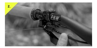
Loosen, but do not remove, the cable fixing bolt on the underside of the dropper lever with a 3mm allen wrench, screw the barrel adjuster fully in clockwise, and make sure the cable housing has a housing end installed. Insert the dropper cable through the barrel adjuster until the housing is completed seated in barrel adjuster, threading the cable under the cable fixing bolt and washer
