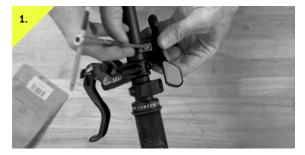
Position hinged clamp on bar and attach lever to clamp using one of the threaded hole options on lever body to achieve your desired position. Tighten with 3mm allen wrench to maximum 2nm. Note: This position can be changed after install to fine tune fit.
