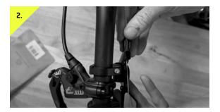
Loosen, but do not remove, the cable fixing bolt on the underside of the dropper lever with a 3mm allen wrench, screw the barrel adjuster fully in clockwise, and make sure the cable housing has a housing end cap installed. Insert the dropper cable through the barrel adjuster until the housing is completely seated in barrel adjuster, threading the cable under the cable fixing bolt and washer.
