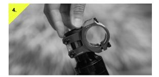
Install your stem with the same number of headset spacers as you noted earlier. Be sure to have at least one 5mm 1-1/8" headset spacer under the stem. Depending on your existing stem stack height, you may need additional spacers above the Loam Stem.
