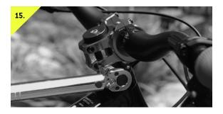
Torque the stem steerer bolts to 6Nm.
