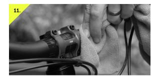
If you used carbon assembly paste, wipe away any excess.
