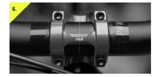
Install the handlebar into the stem and replace the faceplate by loosely and evenly tightening each faceplate bolt. Ensure the faceplate is in the correct position by checking the "PNW" logo on the front is upright.
