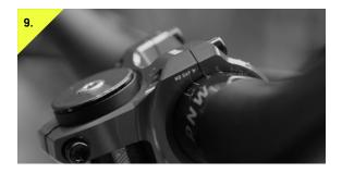
Once the bar is in the correct position, tighten the top two faceplate bolts until there is no gap between the faceplate and the stem body. Torque to 6Nm.
