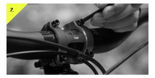
The bar should be held in place, yet still able to rotate easily. Note\* If installing a carbon fiber handlebar, check your handlebar manufacturer's recommendation regarding carbon assembly paste.
