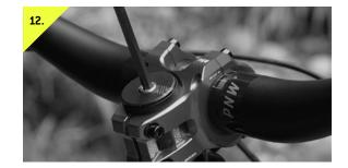
Install and tighten the headset top cap.
