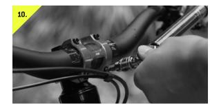
Once the top two bolts are tight, proceed to tighten the lower stem bolts. Torque to 6Nm.
