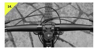
Adjust the bars/stem so that the bars are straight and aligned with the front tire.
