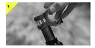
Loosen the Loam stem steerer bolts on your PNW Loam stem so that the stem can easily fit onto the fork steer tube.
