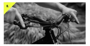
Rotate the bar to your preferred alignment and be sure the bar is in the center of the stem.
