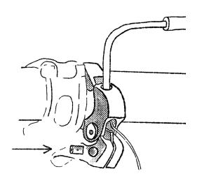
INSERT BARREL NUT INTO THE ROUND FLOATING CENTER
