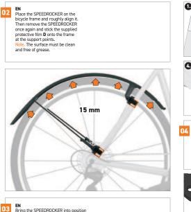
EN Bring the SPEEDROCKER into position and attach it to the seat tube in the first step. To do this, thread the Velcro strap B with the rubberized side facing the seat tube over the protec-tive film and tighten. If necessary, slide the extendable extension profile into the correct position.
