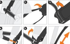
EN Position the SPEEDROCKER mounting adapter on the protective foil. Then thread the enclosed rubber straps B through the opening on the adapter and pull them forward. Then fasten them there via the eyelets.
